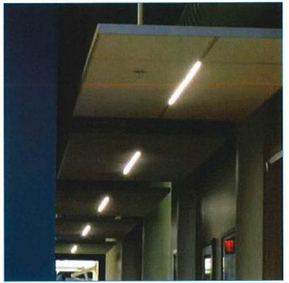
21. The T-BAR LED Smartlight™ product replaces ordinary structures in suspended ceilings and allows the usual florescent light fixtures to be entirely removed.
